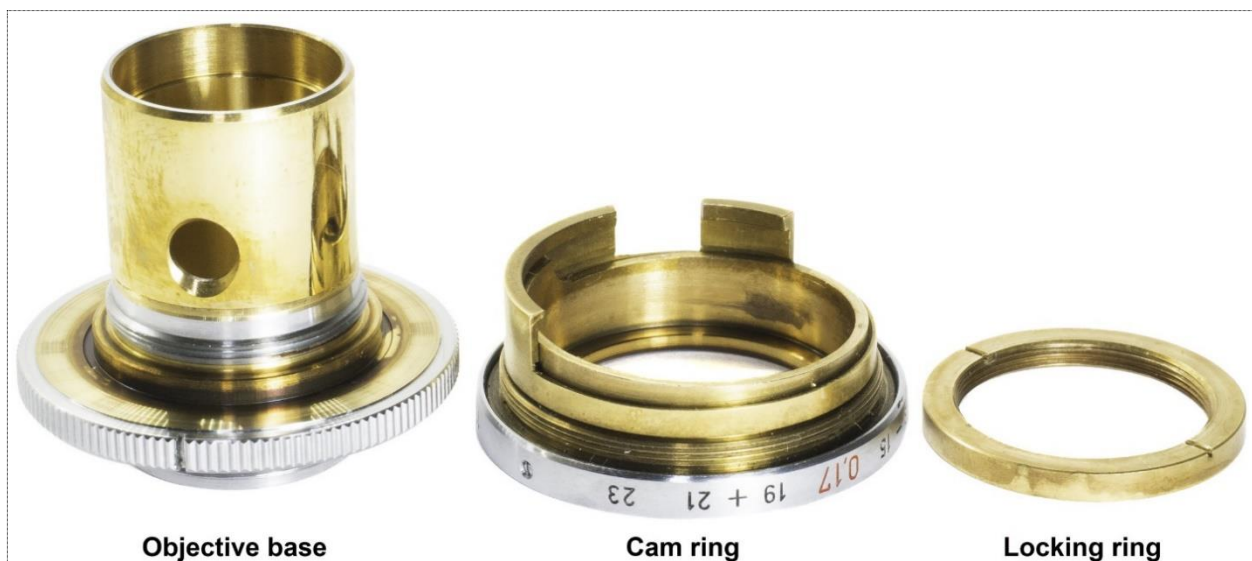
Figure 32: The cam ring removed from the objective base.
