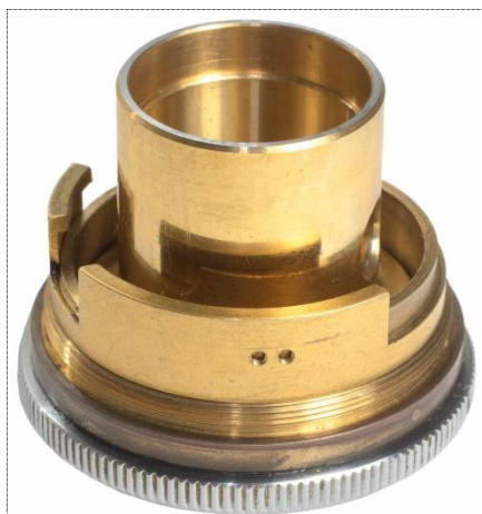
Figure 14: The cam limiter still attached on the cam ring, but with the grub screws removed.
