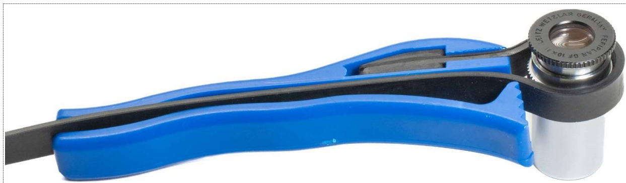
Figure 7: One example of a commercially available strap wrench (jar opener.) Here the strap is wrapped over an eyepiece.
