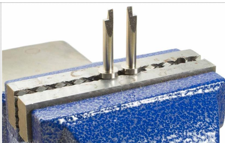
Figure 34: Spanner tips clamped in a heavy vise.
