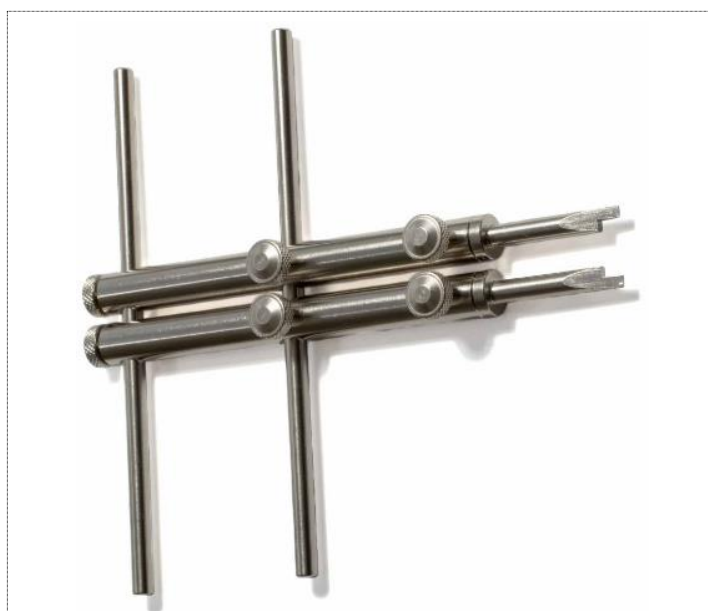
Figure 19: One example of a camera lens spanner with removable tips.
