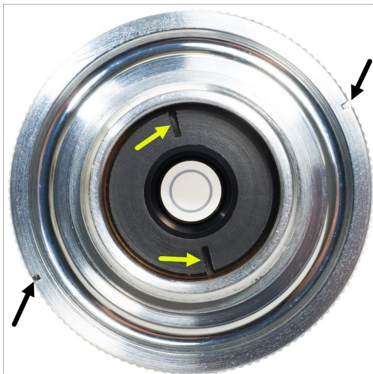
Figure 17: The objective's rear aperture (black) viewed from the mount end of the objective. The yellow arrows point to the spanner grooves. The black arrows point to the index bars for the cover glass thickness scale.
