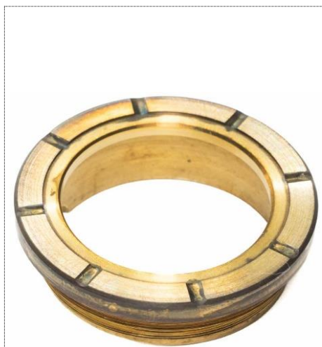
Figure 33: The underside of the cam ring. The 8 grease grooves support the lubrication.
