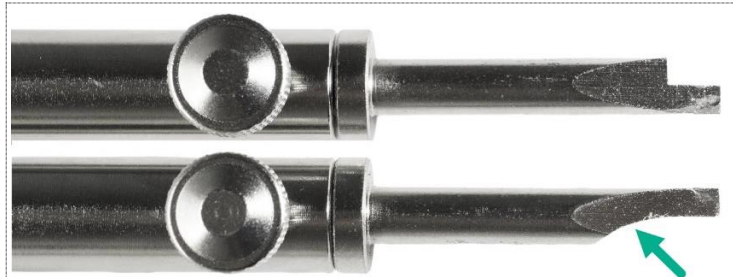
Figure 31: One of the spanner pins ground down.
