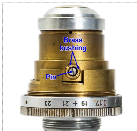
Figure 16: View of the brass bushing with the other pin.
