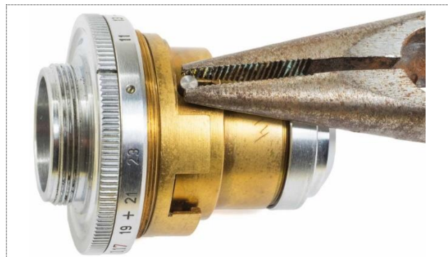
Figure 21: Needle nose pliers holding the cam pin (i.e., pin “A”).
