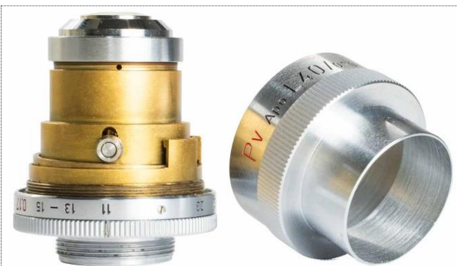
Figure 9: The objective after the barrel has been removed.
