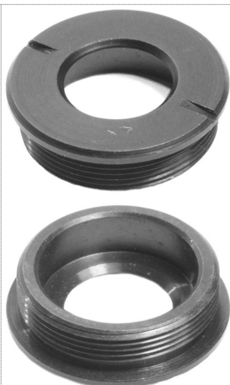
Figure 18: The rear aperture after removal from the inner lens casing.
